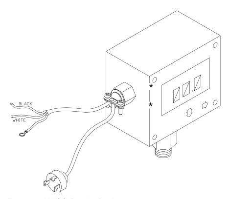
Figure 8-6. L.W.C.O. Electrical Box Assembly
