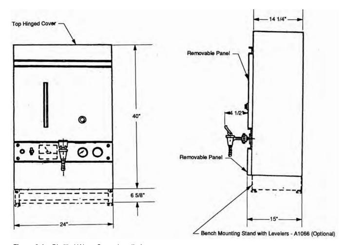
Figure 2-1a. Distilled Water Center Installation
