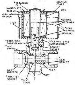
Figure 5-3. 1/2 NPT Auto Drain Valve
