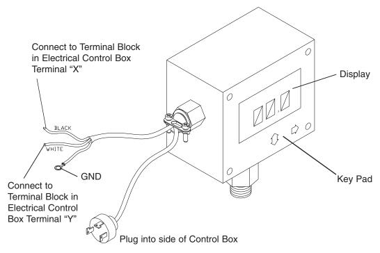
**Figure 5-6.** Level Monitor Installation
