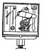
Figure 5-7. Level Monitor - Used on Units Before 2009
