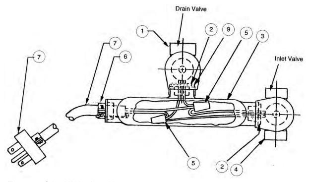
Figure 8-3. Solenoid Valve Assembly
