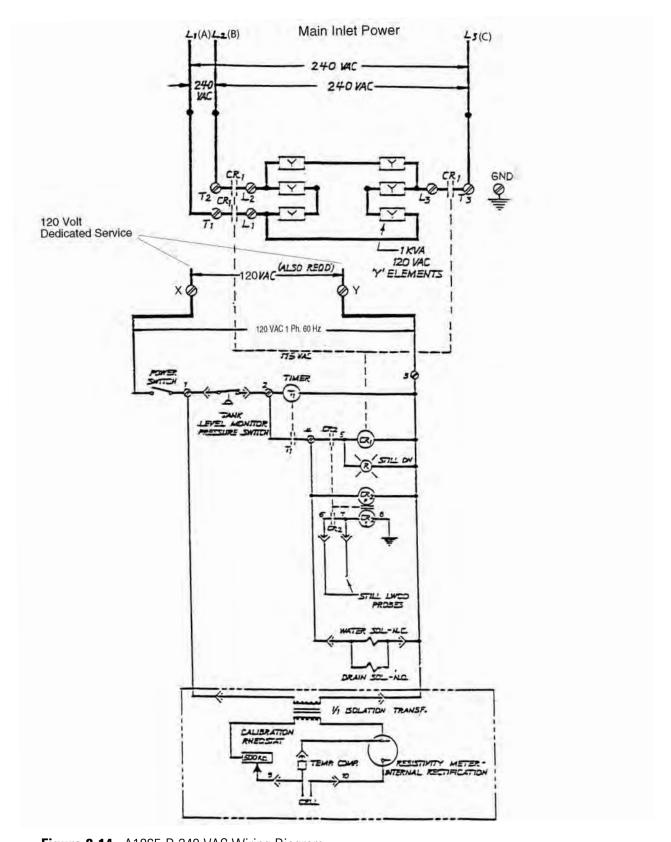
Figure 8-14. A1065-D 240 VAC Wiring Diagram
