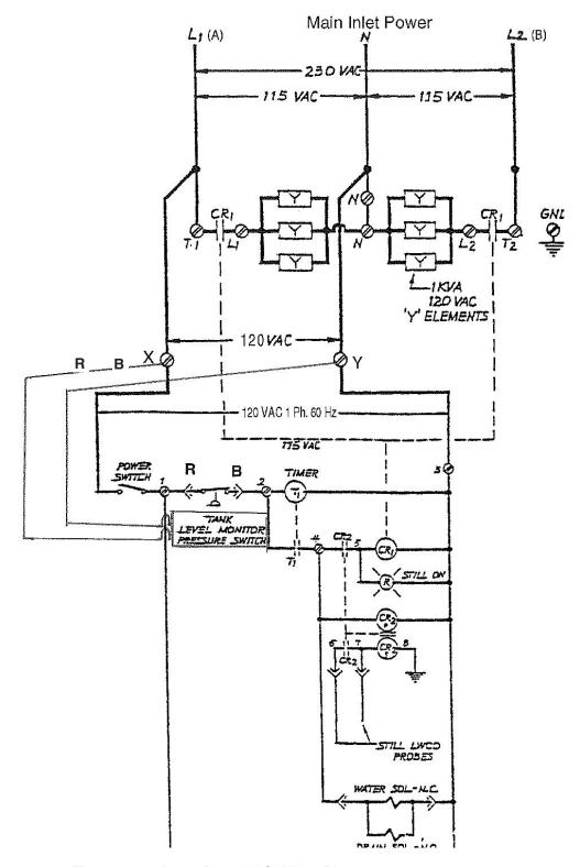
Figure 8-12. A1065-B 230 VAC Wiring Diagram
