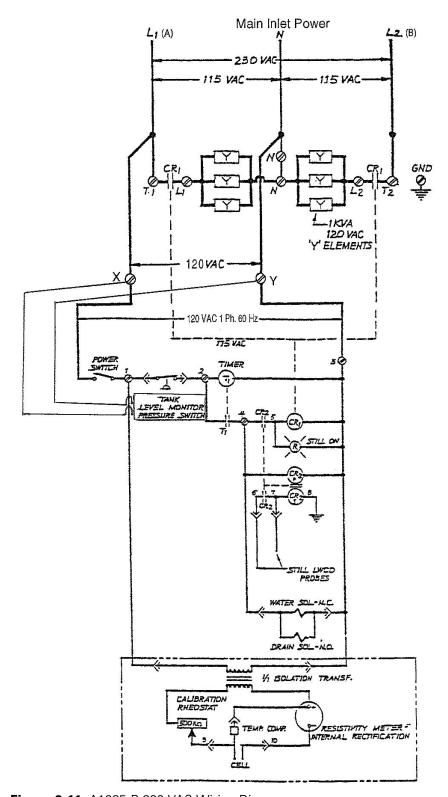
Figure 8-11. A1065-B 230 VAC Wiring Diagram
