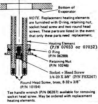
Figure 5-1. Heating Element Replacement
