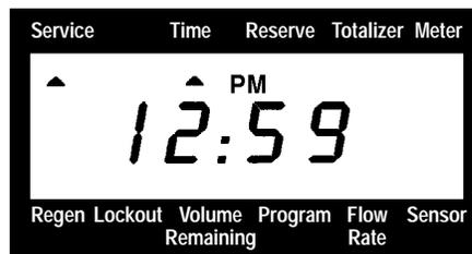
13. *Flow Meter Equipped Valves Only:* The Volume Remaining Display is the volume of water (in gallons) remaining prior to regeneration, including any reserve capacity. Without any water usage the Meter Arrow should be either off or on but not changing. Open a soft water tap. The Meter Arrow should begin flashing at a rate that varies with flow rate. Close the tap after 3 - 5 gallons of water flow.
